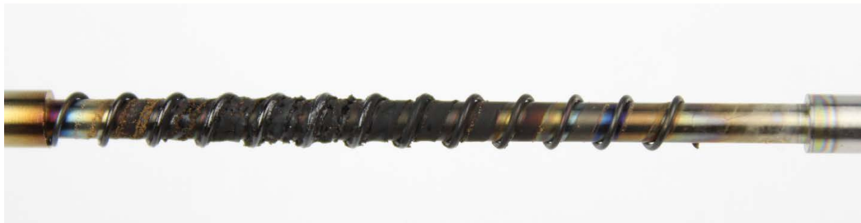
Figure 62: Synthetic oil #5 TEOST MHT rod deposits
