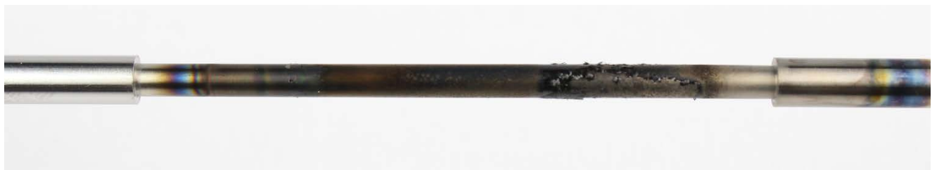
Figure 57: Synthetic oil #2 TEOST 33C rod deposits
