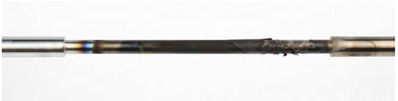
Figure 55: Synthetic oil #1 TEOST 33C rod deposits
