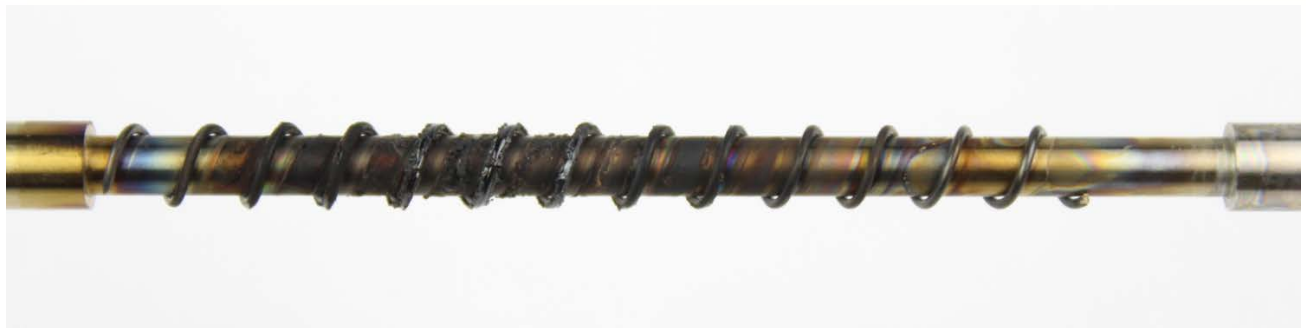
Figure 50: Conventional oil #4 TEOST MHT rod deposits
