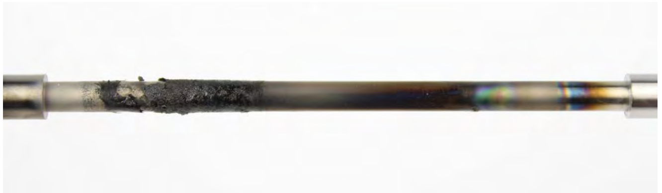
Figure 51: Conventional oil #4 TEOST 33C rod deposits
