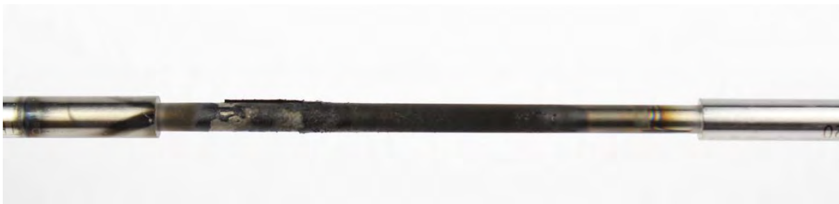
Figure 53: Conventional oil #5 TEOST 33C rod deposits
