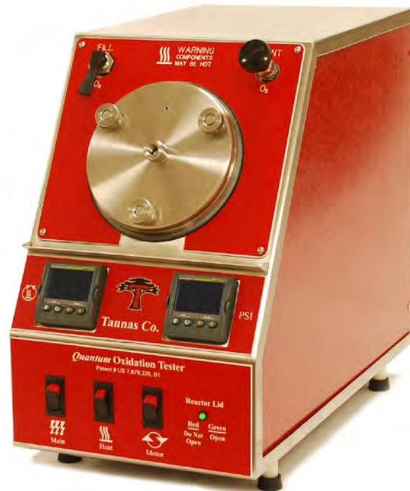
Figure 22: ASTM D4742 TFOUT instrument Image Source: AAA
