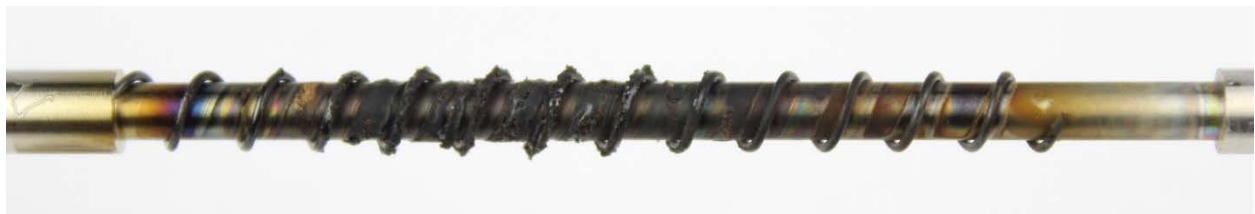
Figure 60: Synthetic oil #4 TEOST MHT rod deposits
