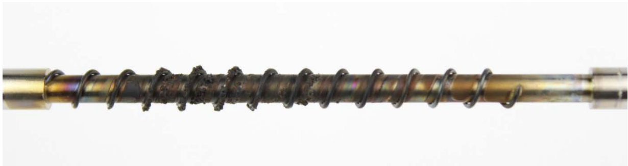
Figure 52: Conventional oil #5 TEOST MHT rod deposits
