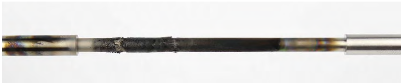
Figure 45: Conventional oil #1 TEOST 33C rod deposits
