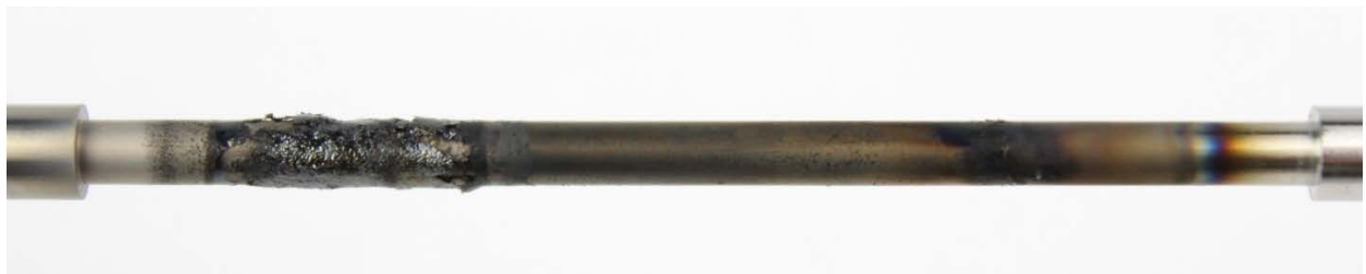
Figure 61: Synthetic oil #4 TEOST 33C rod deposits
