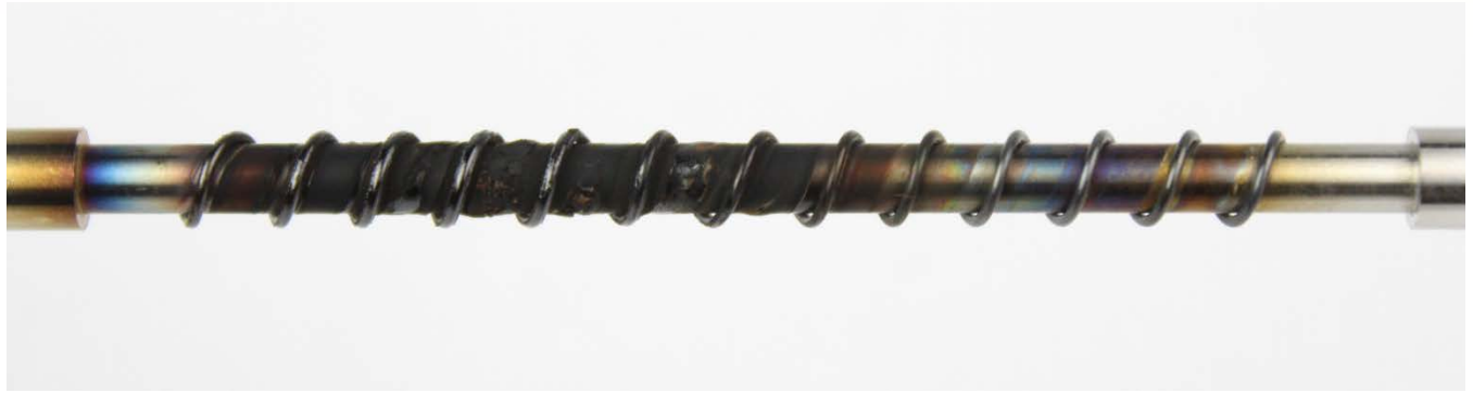
Figure 54: Synthetic oil #1 TEOST MHT rod deposits
