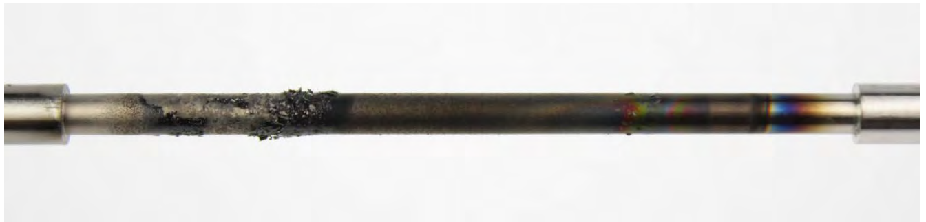
Figure 59: Synthetic oil #3 TEOST 33C rod deposits
