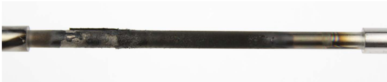
Figure 63: Synthetic oil #5 TEOST 33C rod deposits
