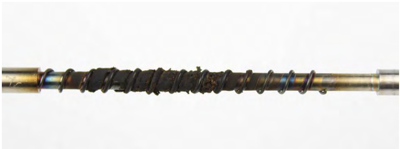
Figure 46: Conventional oil #2 TEOST MHT rod deposits
