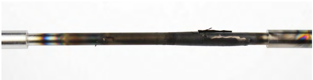
Figure 49: Conventional oil #3 TEOST 33C rod deposits
