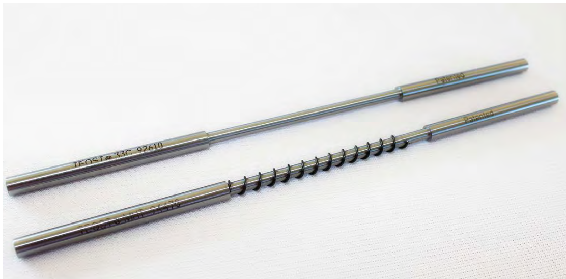
Figure 43: TEOST MHT & 33C depositor rods
