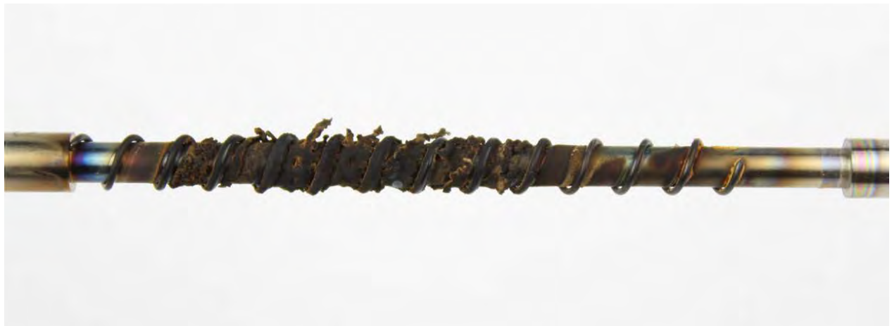
Figure 48: Conventional oil #3 TEOST MHT rod deposits
