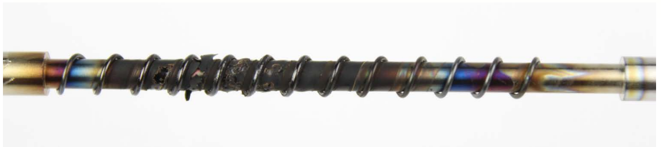
Figure 58: Synthetic oil #3 TEOST MHT rod deposits
