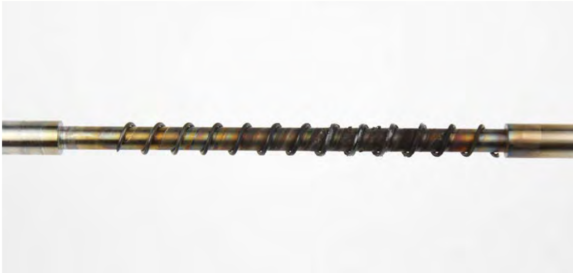
Figure 44: Conventional oil #1 TEOST MHT rod deposits
